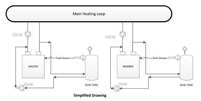
In the above example each DHW tank is controlled individually by a boiler and space heating is provided by both boilers. The Master boiler will be used to provide space heating to the system by using both boilers and DHW heat to its local tank. The Member boiler will provide space heating when called by the Master and DHW heat when requested by its local tank.
