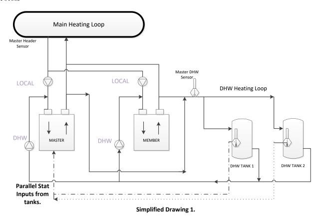
In a (2) loop system, the Master needs to have a Header sensor and a DHW loop sensor attached.
